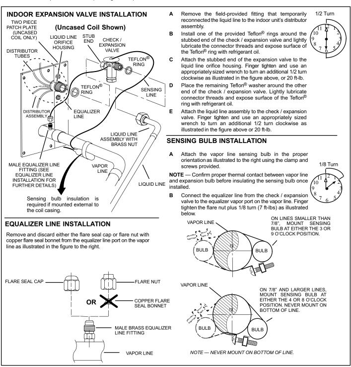
Figure 12. Installing Indoor Check / Expansion Valve
